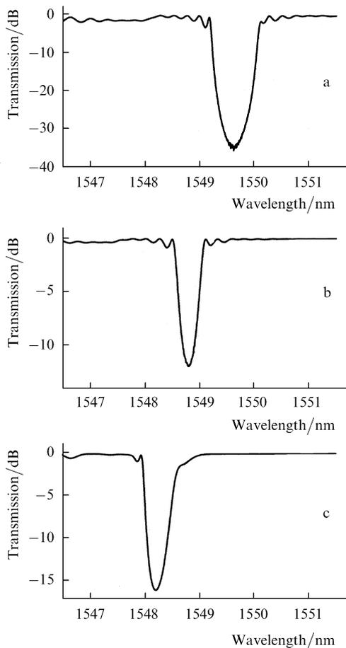
**Figure 1.** Transmission spectra of the FBG for the H<sub>2</sub>-loaded SMF-28 fibre for the pulse intensity  $I = 47 \text{ GW cm}^{-2}$ , the total fluence  $D_{\text{tot}} = 0.68 \text{ kJ cm}^{-2}$  (a) and  $I = 31 \text{ GW cm}^{-2}$ ,  $D_{\text{tot}} = 0.63 \text{ kJ cm}^{-2}$  (b) and for the Nufern GF1 fibre for  $I = 77 \text{ GW cm}^{-2}$  and  $D_{\text{tot}} = 4.7 \text{ kJ cm}^{-2}$  (c).
