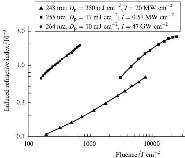
**Figure 3.** Dependences of the induced refractive index on the fluence in the H<sub>2</sub>-loaded SMF-28 fibre irradiated by different lasers ( $D_p$  is the pulse energy density).
